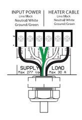
FIGURE 3. Contractor connections.
