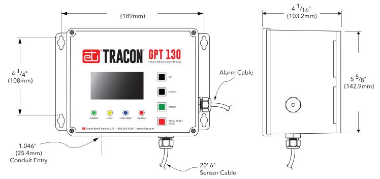
FIGURE 2. Mounting dimensions.
