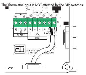
FIGURE 4. Temperature sensor wiring
