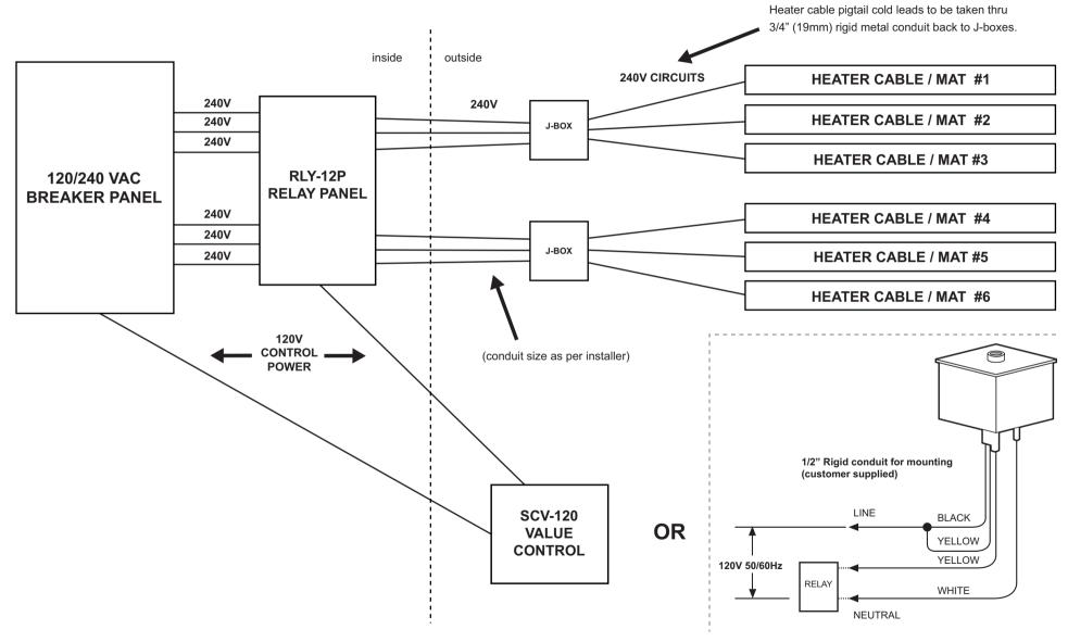
INSTALL IN ACCORDANCE WITH THE REQUIREMENTS OF ALL APPLICABLE ELECTRICAL AND BUILDING CODES AND REGULATIONS. ENSURE THAT ALL CONDUIT/CABLE TERMINATIONS ARE WATERTIGHT.
